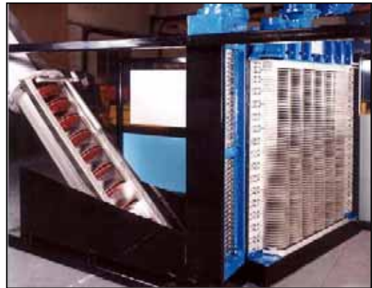
Screw Extraction Package Up to 13,900m 3 /h
